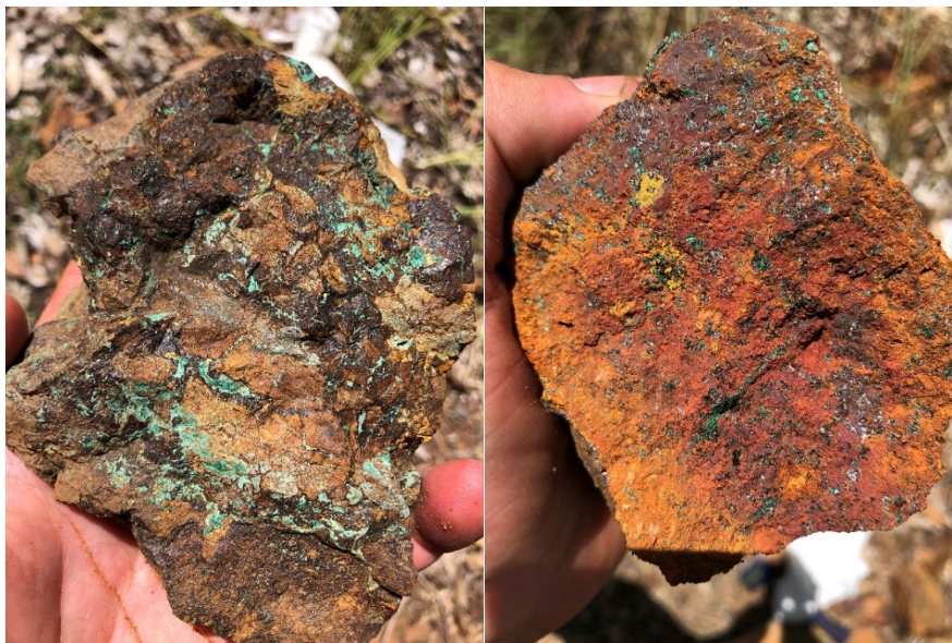
Figure 3: Outcropping Chianti gossan samples with Malachite (L) (GDA94 MGA Z51 611890E, 8167100N) and malachite and chalcocite (R) (GDA94 MGA Z51 611890E, 8167115N)
