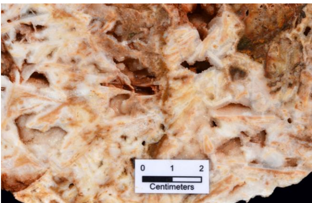
Photo 7: Sample KRS2060076, hydraulic vein breccia with intensely limonite-haematite oxidized wallrock flooded by mesocrystalline quartz after coarse lattice bladed calcite indicating pronounced boiling. 0.28g/t Au at Phoenix Vein Zone.
