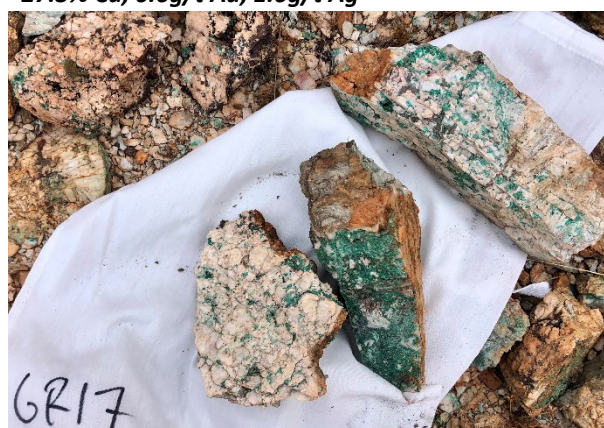
Figure 9: Sample GR17, Quartz and malachite vein. (GDA94 MGA 628909E, 8168420N) 4.2% Cu, 0.1g/t Au, 1.3g/t Ag
