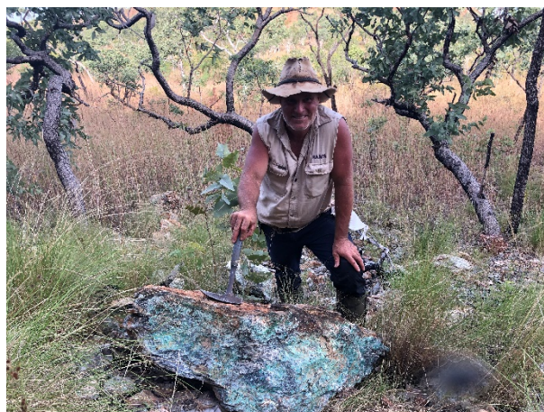
Figure 5: Dreadnought's Drew Money with a massive copper lode of malachite quartz copper oxides and gossanous iron oxides. (GDA94 MGA 628776E, 8168261N) Near Sample IDs GR36, 37, 40
