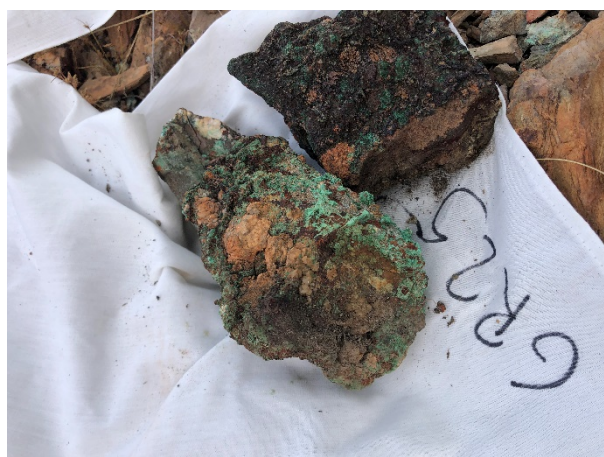
Figure 7: Sample GR25, Quartz with malachite and copper oxides. (GDA94 MGA 628874E, 8168360N) 27.3% Cu, 0.6g/t Au, 1.6g/t Ag
