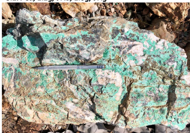
Figure 8: Sample GR20, Silicified slate with quartz veining and malachite. (GDA94 MGA 628903E, 8168397N) 12.4% Cu, 0.2g/t Au, 1.7g/t Ag
