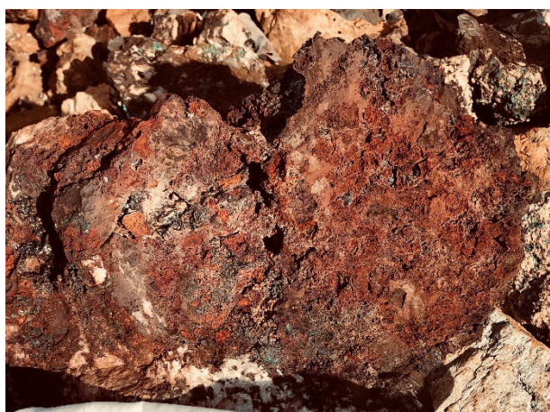
Figure 6: Sample GR19, Gossanous ironstone with trace malachite. (GDA94 MGA 628909E, 8168420N) 3.2% Cu, 1.2g/t Au, 1.0g/t Ag
