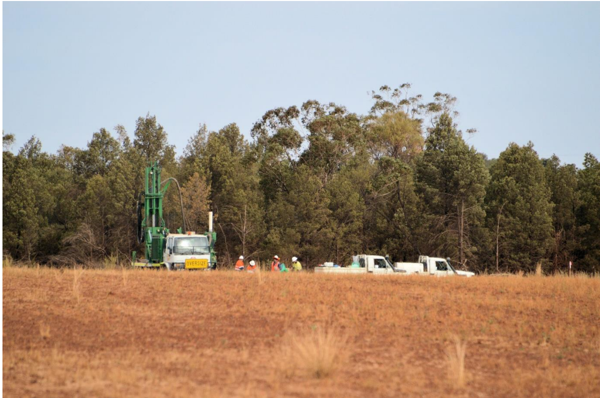
Figure 3: Photo taken of air core drilling rig in operation during Australian Mines' May 2019 resource expansion drill program at its Flemington Project in central New South Wales.
