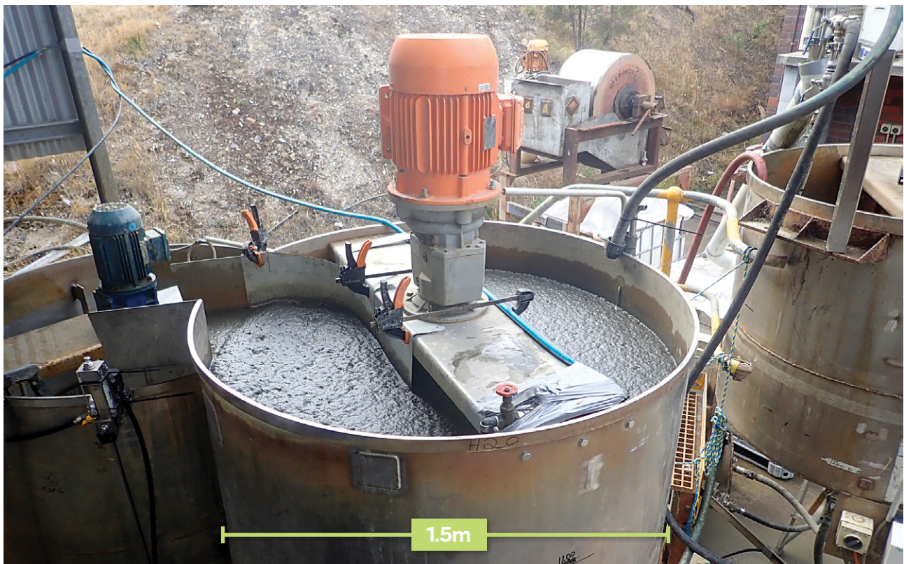
Figure 5. Operating float cell, with pyrite collected in the froth at the top of the cell.
