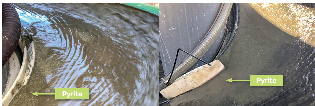
Figure 4. Operating rougher spiral (LHS) and cleaner spiral (RHS), with 'heavy' pyrite concentrate being separated from 'light' feldspar/silica gangue.
