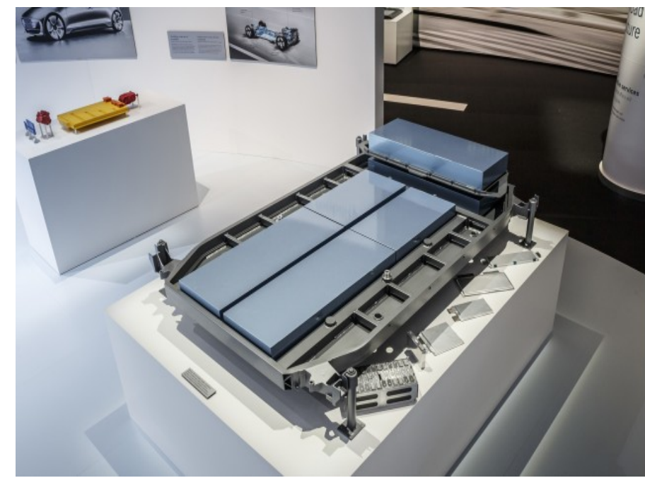
↑ Mercedes Benz NMC lithium-ion battery prototype
