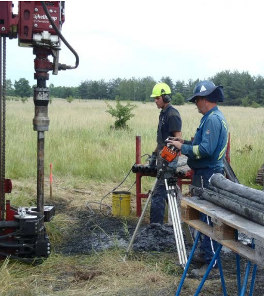
↑ Sonic drill – modern, effective sampling tool
