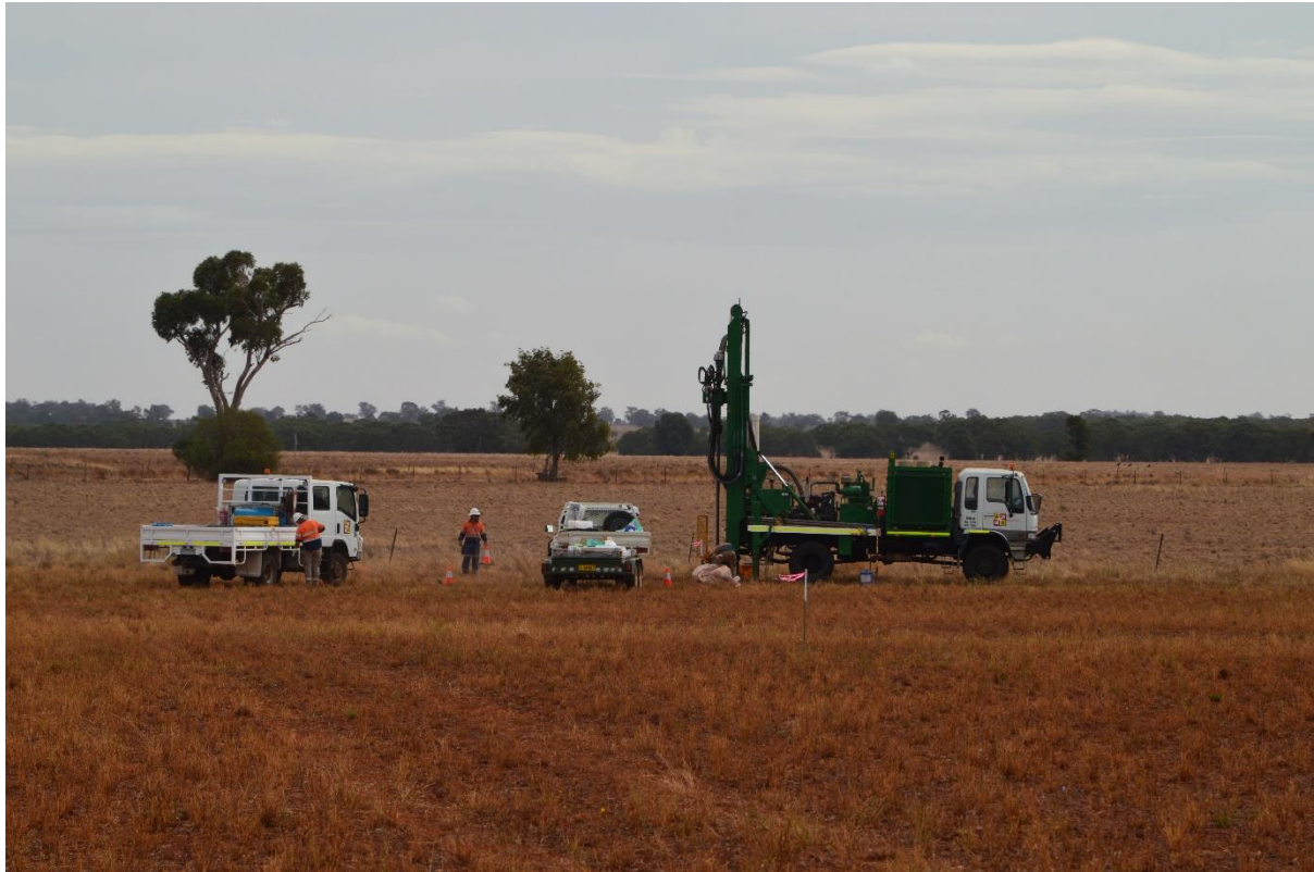
Figure 3: Photo taken of aircore drilling rig in operation during Australian Mines' May 2019 Mineral Resource expansion drill program at its Flemington Project in central New South Wales.
