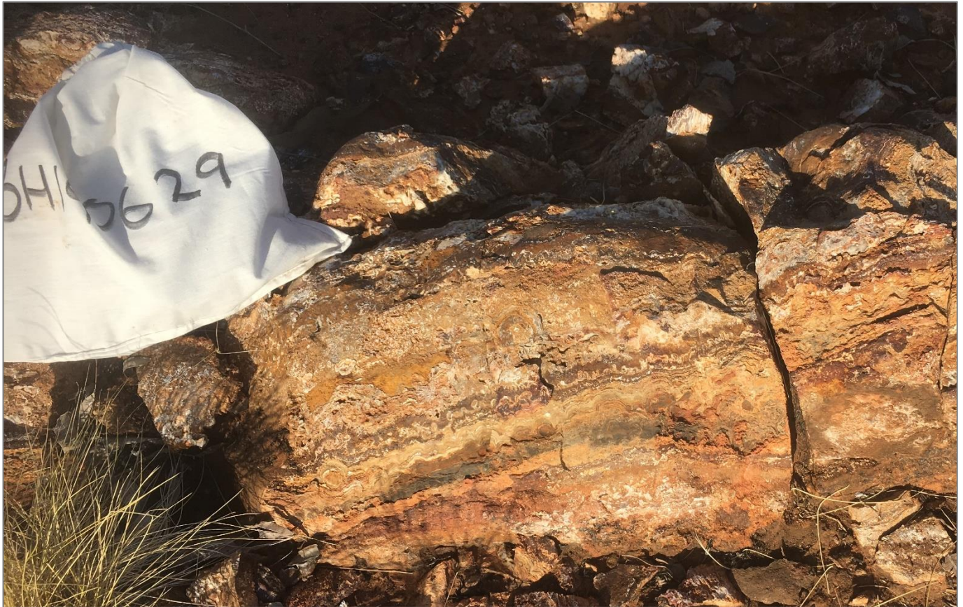
Figure 4: Photo taken at the site of sample BH190629 showing colloform banded sulphide textures. This sample returned an assay value of 24.2% zinc and 62.2 g/t silver. Width of photo ~ 1 metre.
