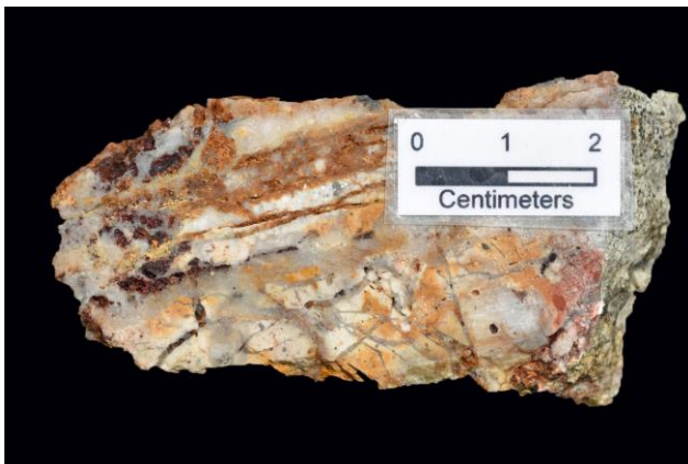
Photo 5: New Outcrop Sample KRS206353, 14.3g/t Au and 1190g/t Ag . Intensely silica-illite/adularia-pyrite altered and limonite-haematite-stained, hydraulically brecciated and interlocking crystalline quartz network rehealed dacitic to rhyolitic lithic-lapilli tuff. Limonite and haematite are after oxidised sulphides. Bonanza Zone.
