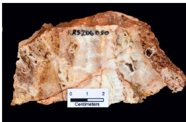
Photo 9: Sample KRS206030, polyphasal hydraulic breccia comprised of limonitic to haematitic ripped up wallrock fragments set in a mesocrystalline to interlocking crystalline quartz-adularia and cut through by crystalline interlocking quartz. 1.67g/t Au, 1.1g/t Ag at Golden Palm vein corridor.
