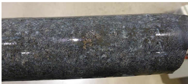
FIGURE 15. MINERALISED PORTION OF NQ DRILL HOLE KMD-07-01 AT 326.6M DOWNHOLE
