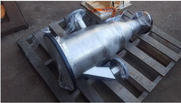
The upgraded EVAP plenum pre-installation
