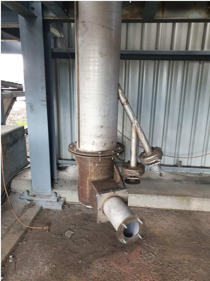
The lower body of the upgraded FB Roaster with plenum installed
