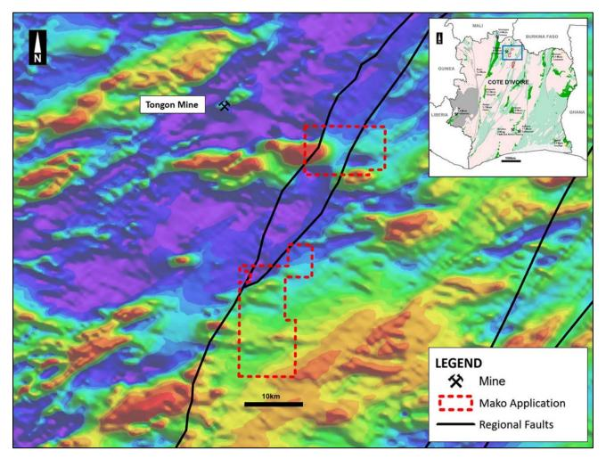
Figure 2: Regional magnetic geophysics (RTP) with Mako permit applications
