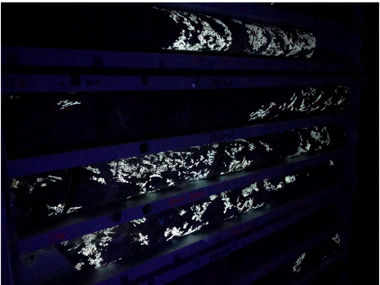
Figure 1: Photograph of portion of the metallurgical core sample under ultraviolet light (highlighting scheelite mineralisation)
