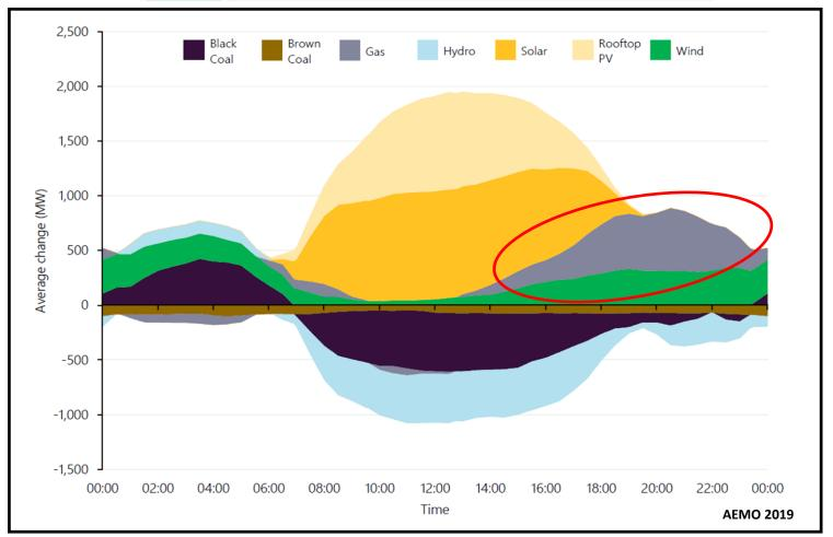
Shift in NEM power generation source... from Q1 2018 to Q1 2019 Black Coal and Hydro displaced by rooftop and grid solar
