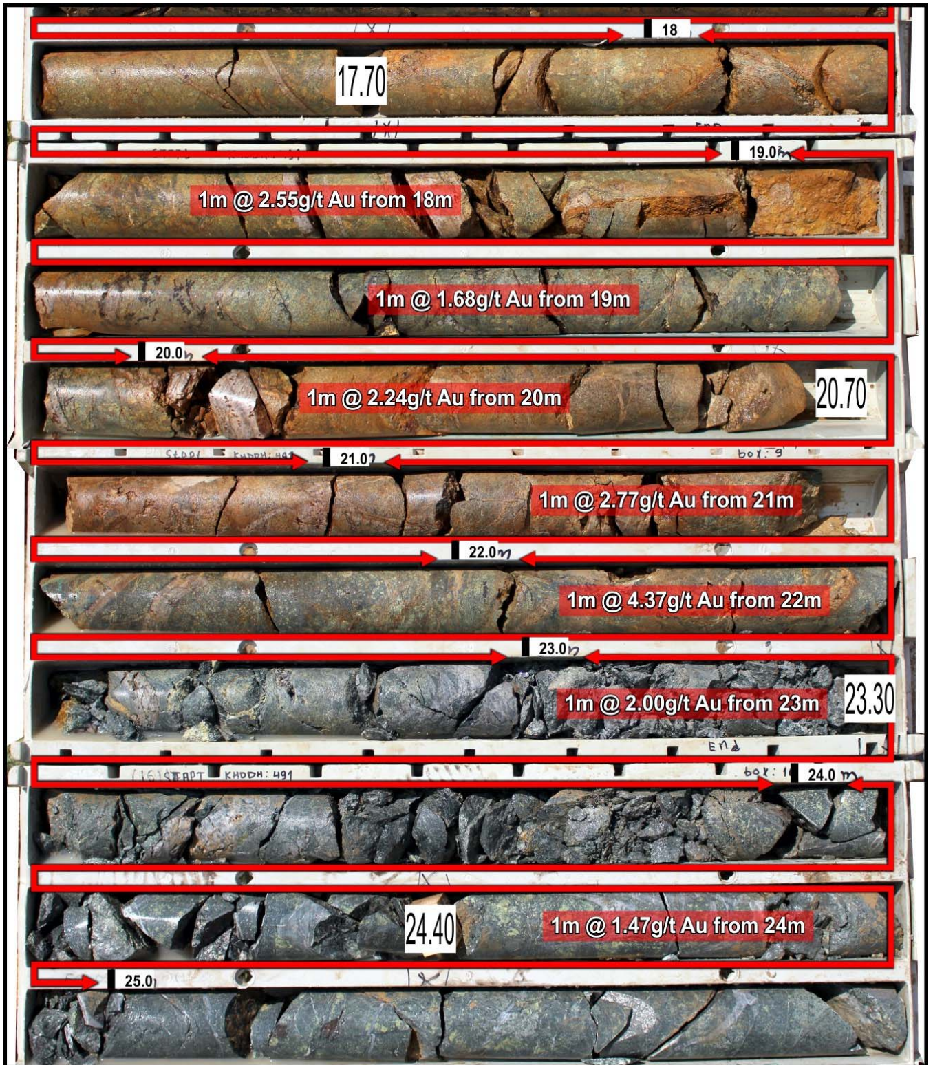
FIGURE 6: Core photographs from KHDDH491 showing the high-grade zone of 15m grading 2.88g/t Au from a depth of 18m to 25m downhole.
