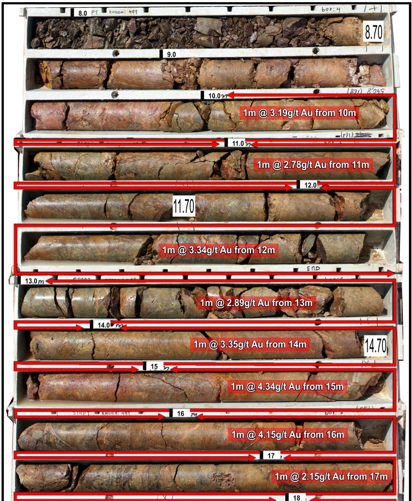
FIGURE 5: Core photographs from KHDDH491 showing the high-grade zone of 15m grading 2.88g/t Au from a depth of 10m to 18m downhole.
