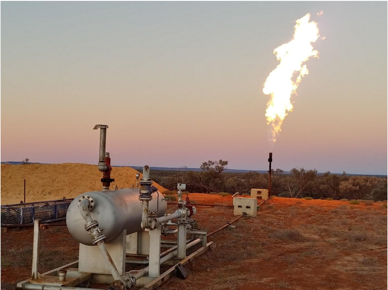
Figure 1: Flow testing operations on Tamarama 2 well
