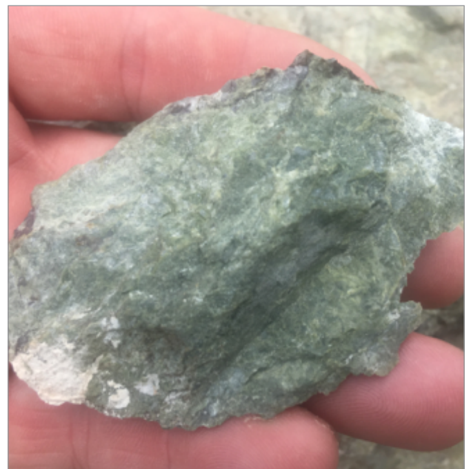
Figure 5. Hand specimen of pervasive epidote (rare earth-rich allanite) mineralisation.
