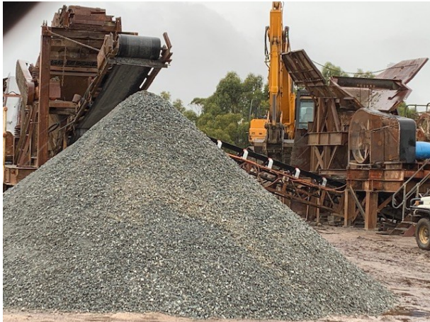
Figure 1a – Stockpile of crushed high-grade skarn material at the Granville East Mine
