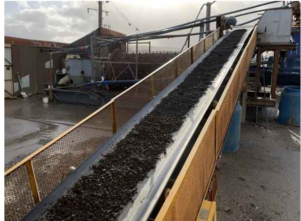
Figure 1b – Crushed high-grade skarn material being fed into the ball mill at the Granville Processing Plant
