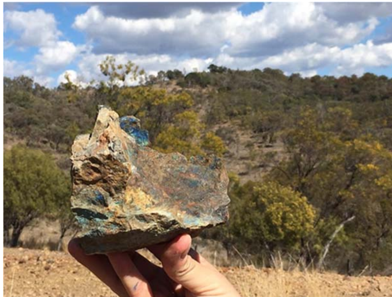
Figure 2 – Reids rock chip sample (assayed 5.79%Cu, 212g/t Ag, 1.24%Zn, 179ppm In and 0.11%Sn) with Taronga Tin Deposit in background
