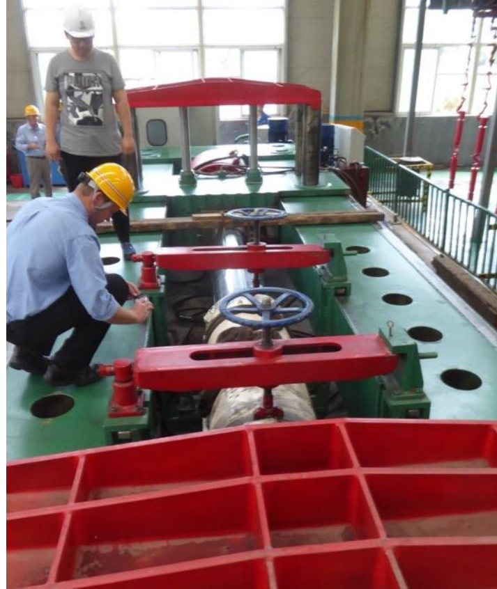
Prototype Leg Cylinder in second test rig undergoing Eccentric cyclic testing
