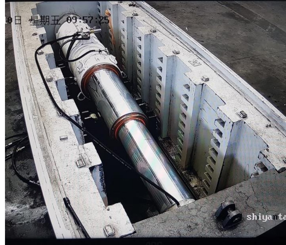
Prototype Leg Cylinder in test rig undergoing standard cyclic testing over 480bar yield range
