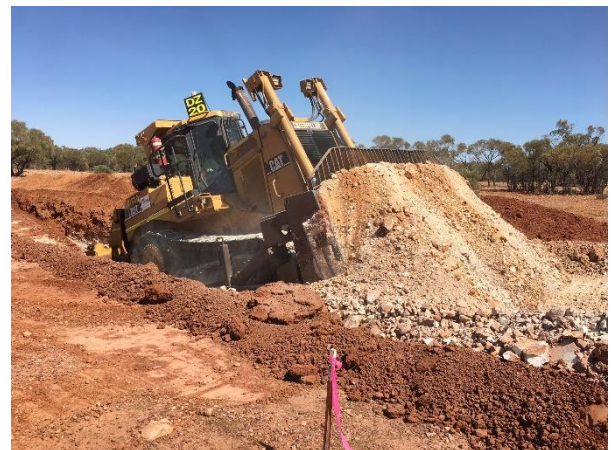
CAPTION: D9 dozer undertaking trial stripping of shale overburden at Ardmore.
