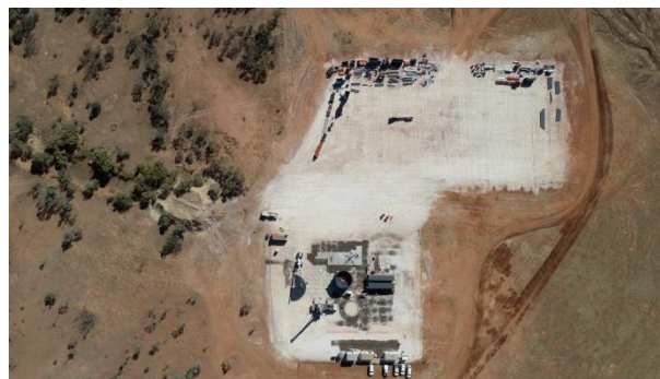
CAPTION: Aerial photograph of site civil works at Ardmore in preparation for plant installation, ROM and concentrate drying pads.
