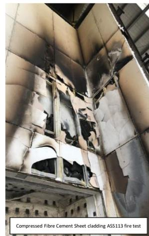
Compressed Fibre Cement Sheet cladding AS5113 fire test
