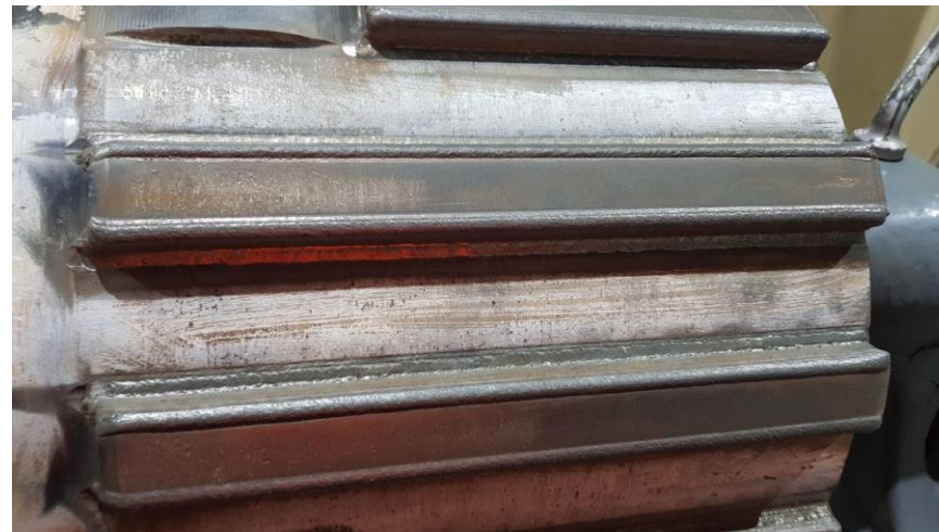
Splines after LaserBond® reclamation before final machining
