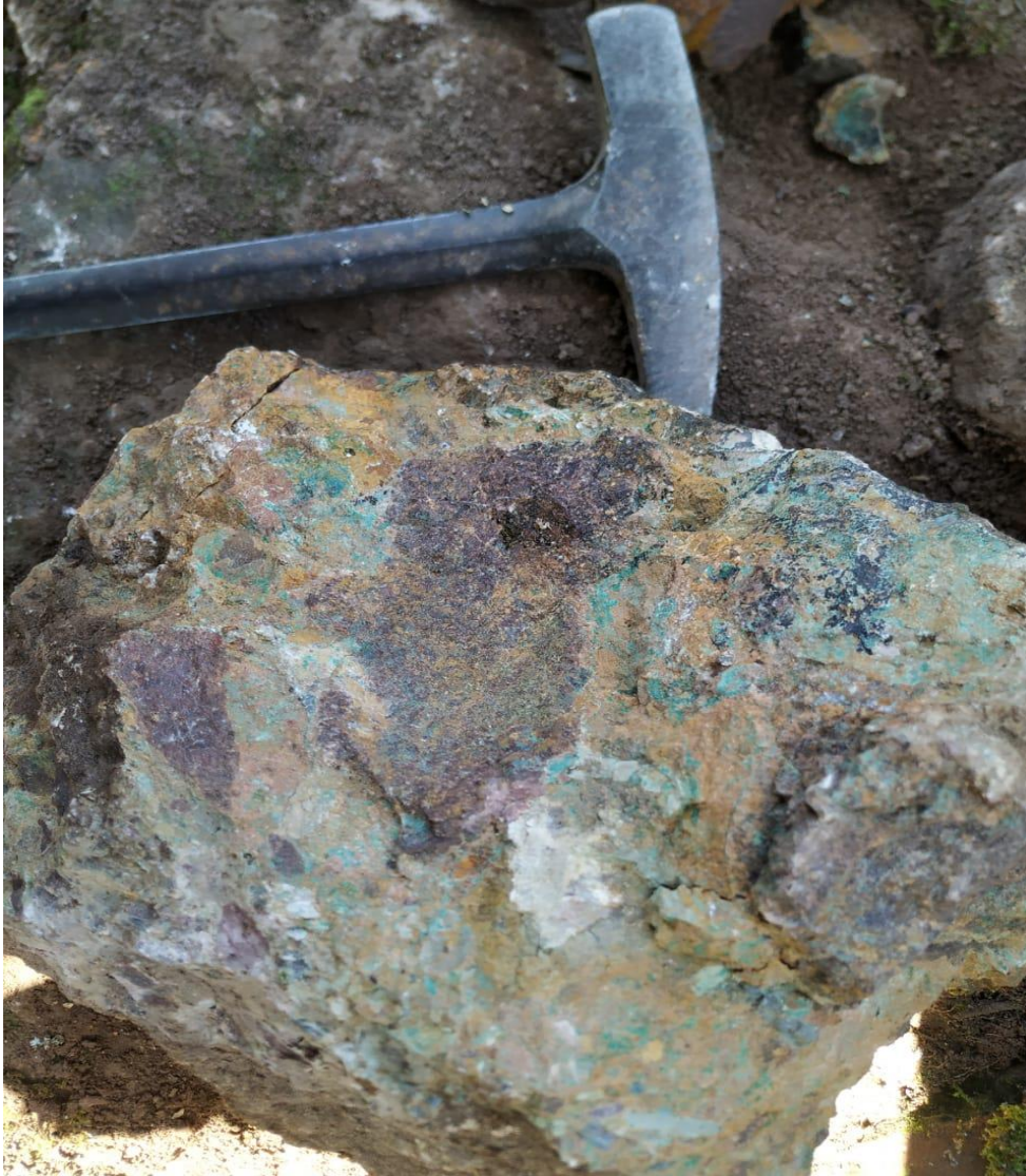
Figure 8 Example of Coarse Conglomerate showing Copper as Malachite within the Weak Porous Matrix between Rock Fragments
