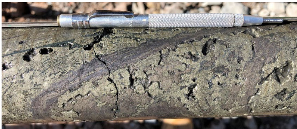
Figure 1: Massive sulphide (photo of interval 61.6m – 61.8m) consisting of chalcopyrite, pyrrhotite, sphalerite and pyrite.
