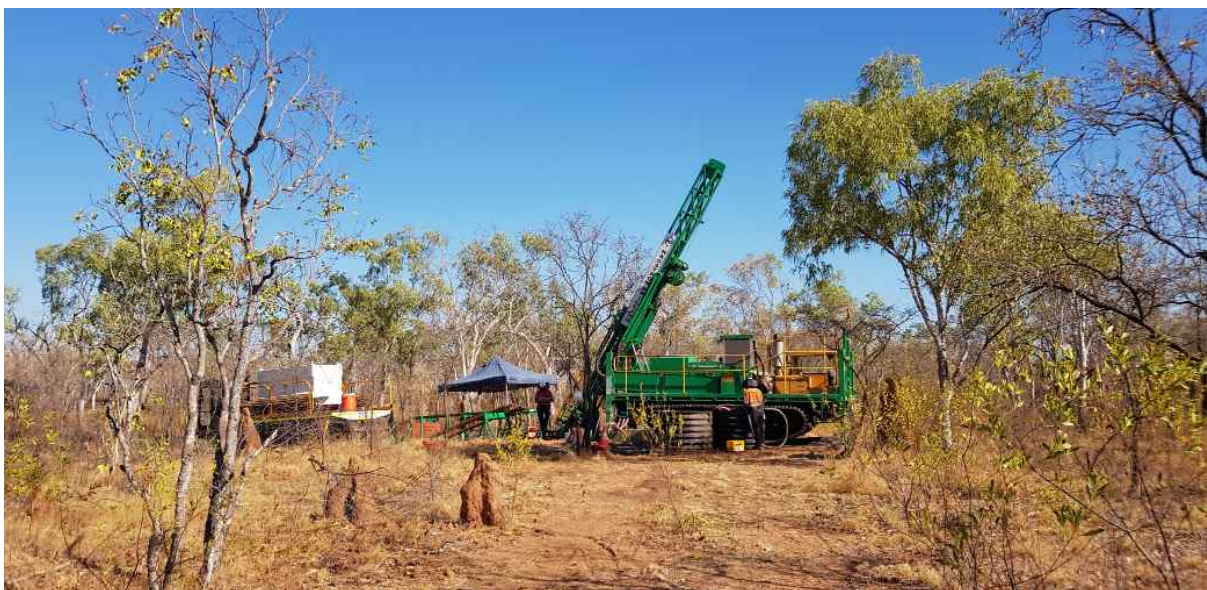
Figure 4: Small footprint diamond rig set up at Chianti drilling CHDD001.
