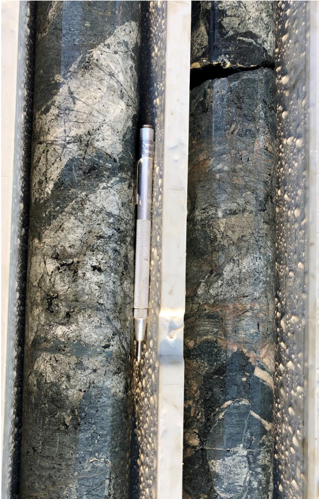
Figure 6: Intense alteration in the stringer zone with chalcopyrite, pyrrhotite and pyrite
