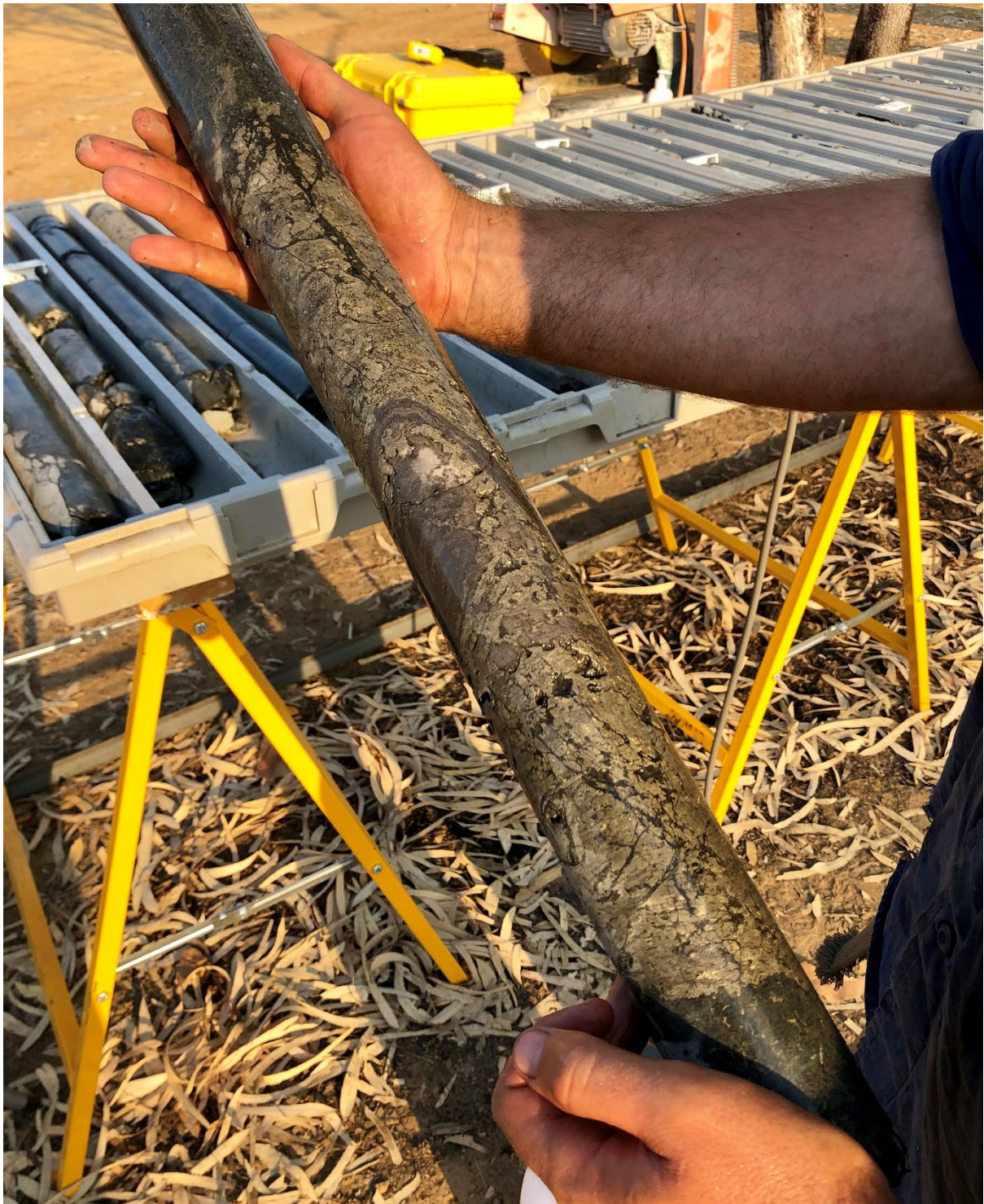
Figure 5: Massive sulphide from 61.5m including chalcopyrite, sphalerite, pyrrhotite and pyrite.
