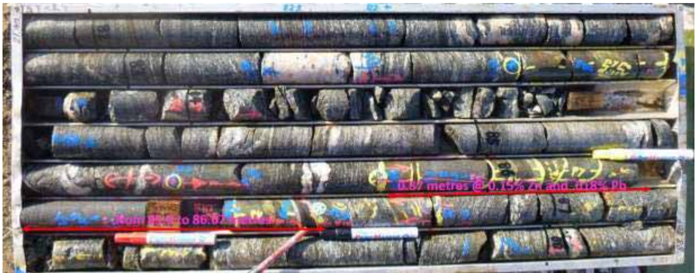
Figure 7: Mineralised garnet & BIF bearing BHT Lode Zone 2 from 85.5 to 86.9 metres.
