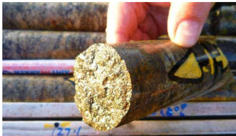
Figure 4: An example of the strongly pyritic (locally cobaltiferous) bands in albitic gneiss in DD95STV3.
