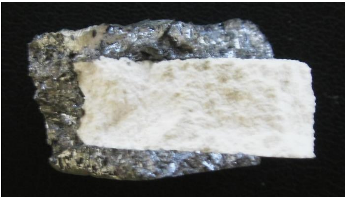
Figure 3. Initial attempted infiltration of mullite preform
