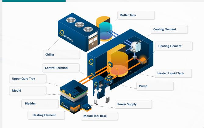
Pictured: Quickstep proprietary Out Of Autoclave (OOA) composite curing technologies.
