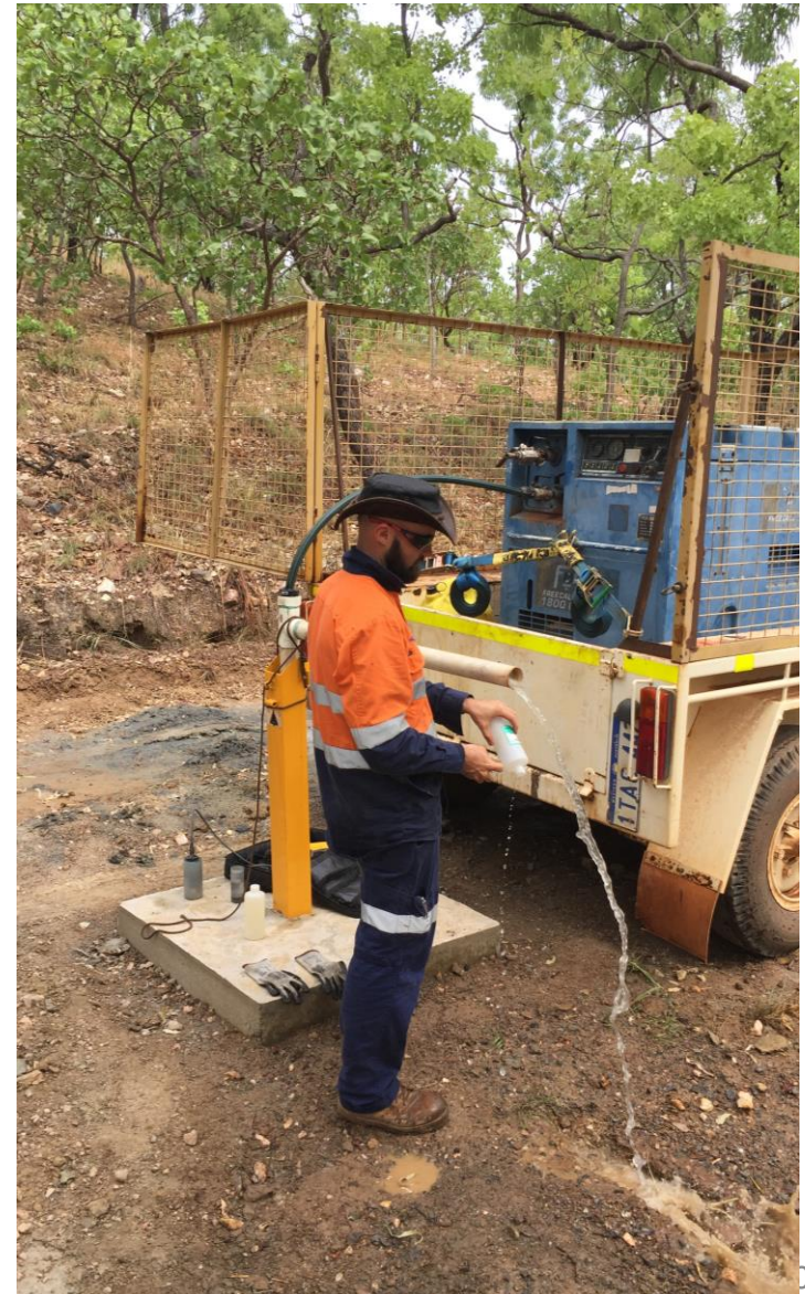
Water bore sampling for hydrological analysis
