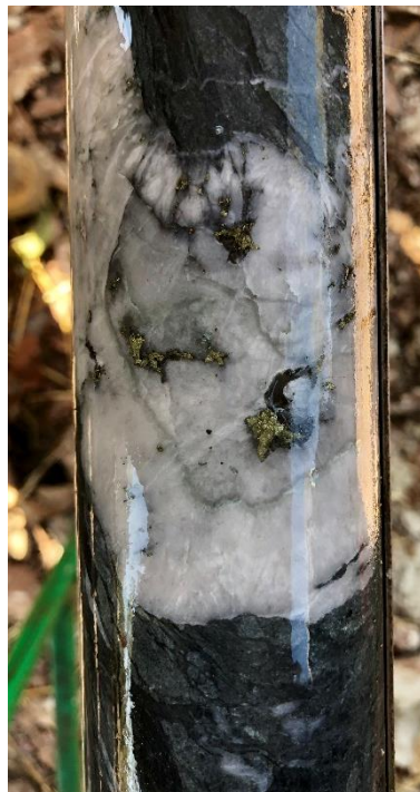
Figure 4: GRDD001 ~28.5m showing a quartz-chlorite-chalcopyrite bearing combed crustiform vein within a highly altered breccia.
