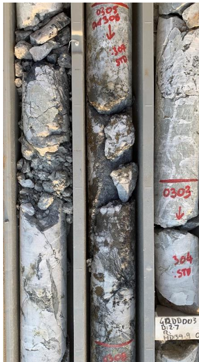
Figure 3: GRDD001 ~39.5-42.5m showing brecciated quartz-pelite zone with intense silica alteration and disseminations / patches of chalcopyrite and chalcocite.
