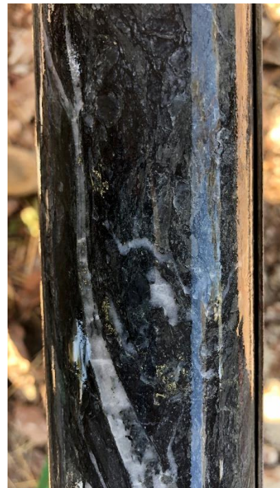
Figure 5: GRDD001 ~27.9m showing disseminated chalcopyrite and pyrite in both the matrix of a highly altered breccia and as infill in quartz veins.
