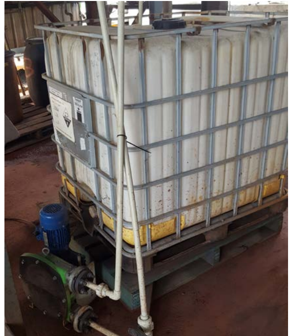
SPL is pumped from the IBC tank into the EVAP fluid bed in the process tower
