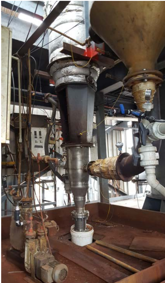
EVAP Fluid bed and plenum prior to insulation
