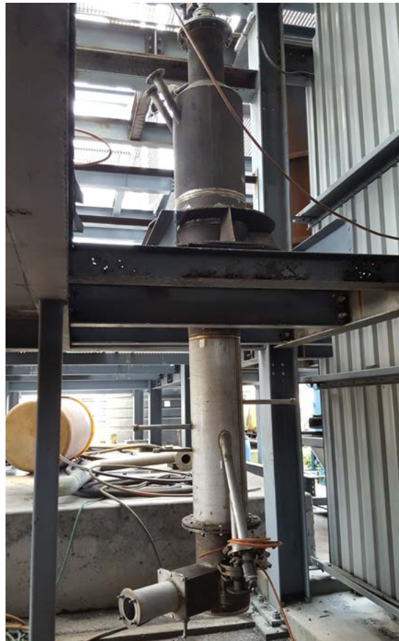
PYRO-FBPR fluid bed roaster prior to insulation
