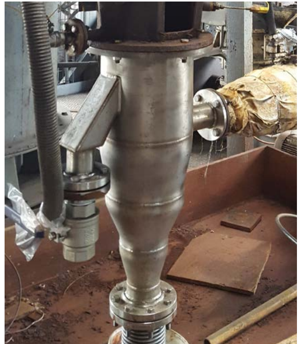
EVAP plenum showing the chloride pellet discharge chute (lower LHS)
