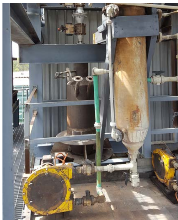
PYRO-FBPR fluid bed roaster prior to insulation
