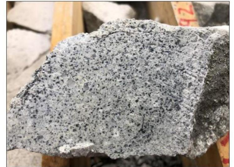
LMDD004 at 68.18m showing black chalcocite and bornite (copper sulphide species) spots through vuggy silica and clay altered volcanic rocks in a 'high sulphidation system'. The interval 68 – 69.6m returned assays of 1.11% copper, 0.2g/t gold, and 5.4g/t silver.
