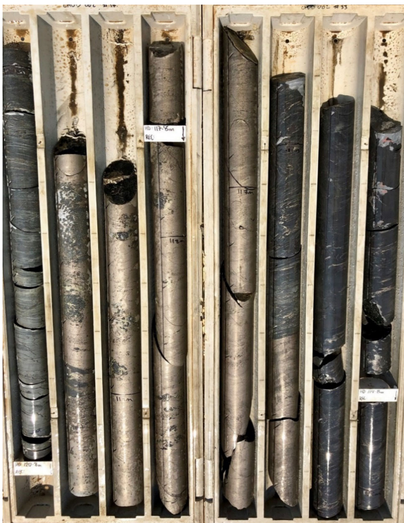
Figure 5 Massive sulphides in the Lower Zone of CHDD002 (po, cp, sp)
