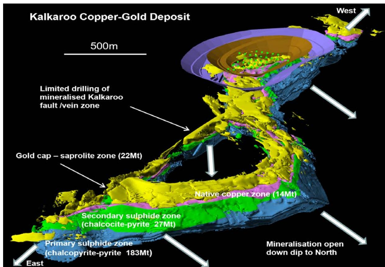
Oblique view of the Kalkaroo copper-gold deposit showing the different ore zones with increasing depth. The mineralisation is open down dip and along strike.
