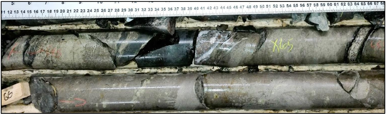
Figure 2: ZA-19-06 - massive sulphide comprising 95% pyrrhotite and 5% chalcopyrite at 65-66.5m downhole.
