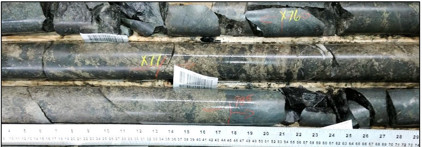
Figure 3: ZA-19-06 - footwall gabbro with semi-massive and net-textured pyrrhotite + pyrite at 76 to 78.5m downhole
