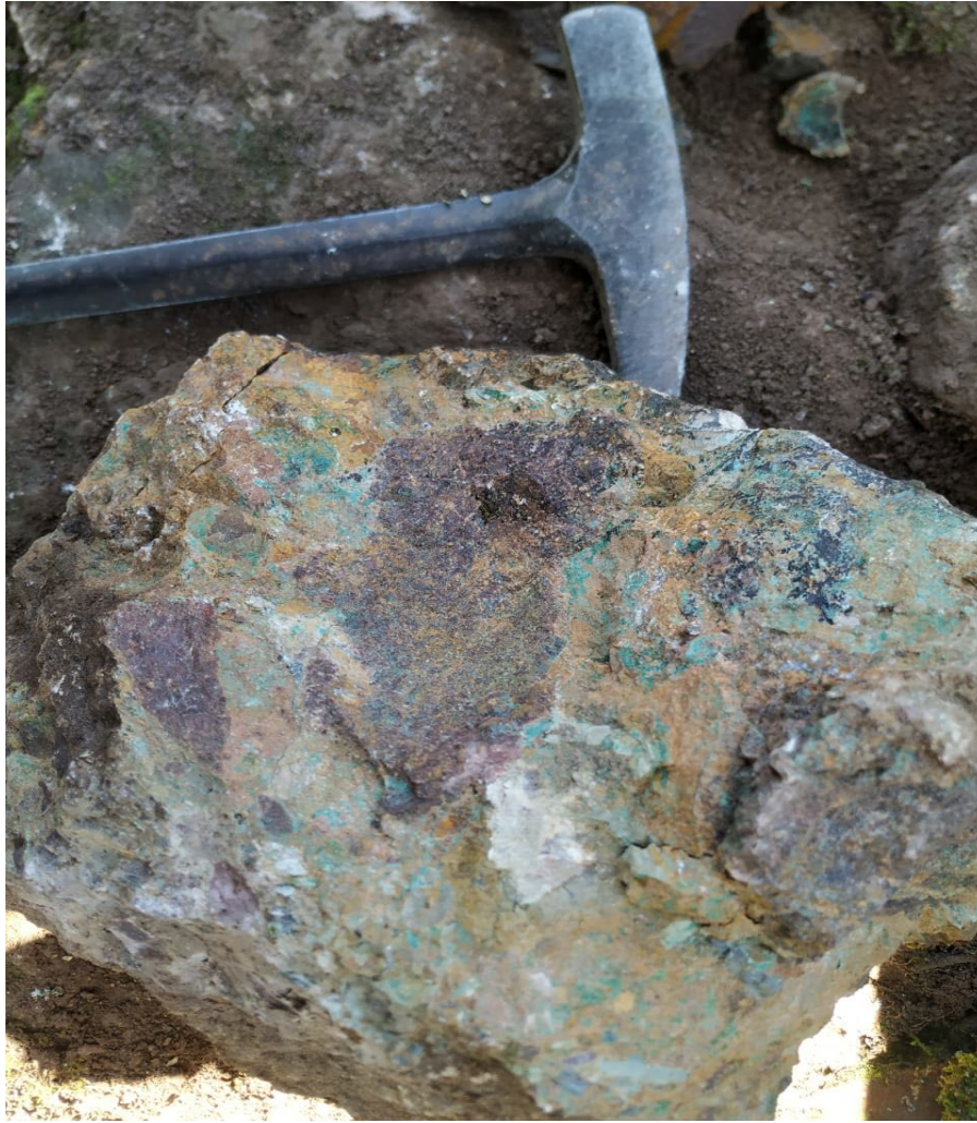
Figure 6 Photo showing the Passo Feio Conglomerate with Abundant Malachite in the Matrix
