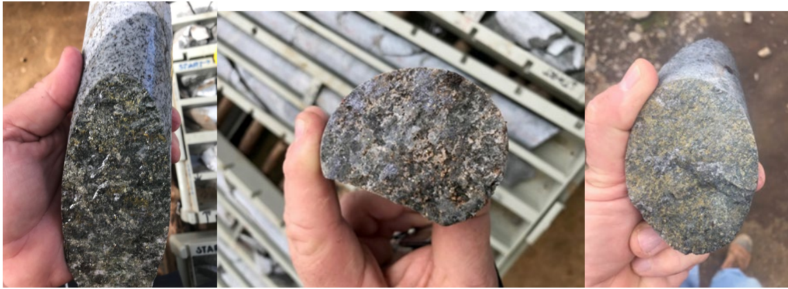
Figure 2; Samples of fracture-controlled mineralisation in MCD003 – Monoyal Prospect
