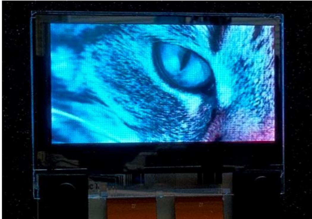
X-Celeprint demonstrates a 2000 cd/m<sup>2</sup> microLED display using RPCVD p-GaN: showing good colour uniformity, quantum efficiency, and forward voltage.
