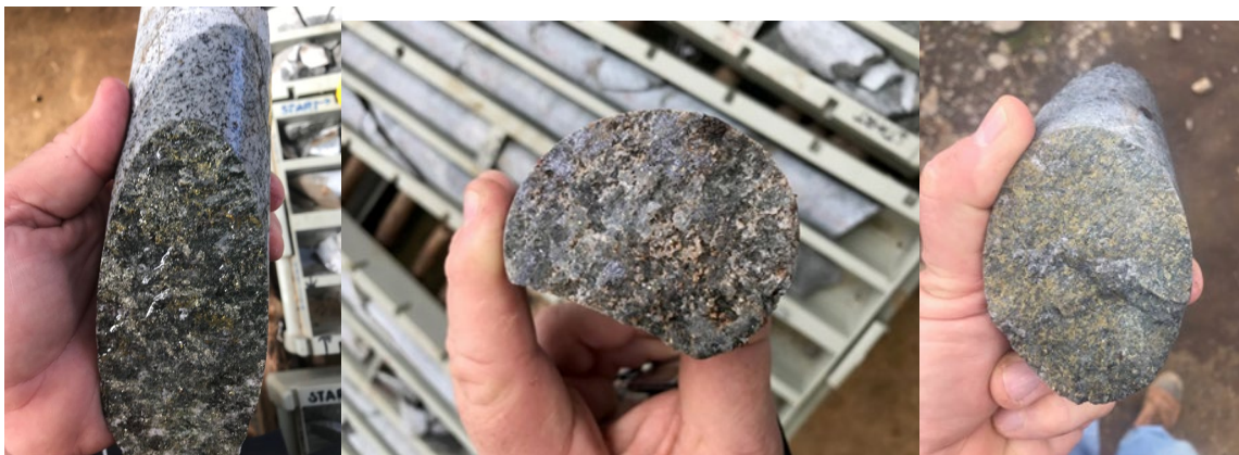
Figure 2. Fracture-controlled sulphide-mineralisation on fracture surfaces in MCD003. From left to right; 30% precipitated sulphides at 271.20m depth, 45% sulphides at 243.20m depth and 55% finely disseminated sulphides at 399.80m depth.
