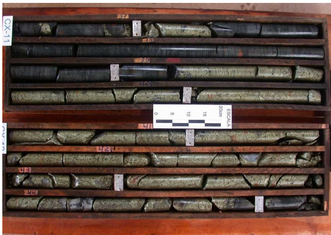
Figure 2: Core photo from drillhole SLUCFD009, displaying the main copper sulphide mineralisation intersected in historical drilling
