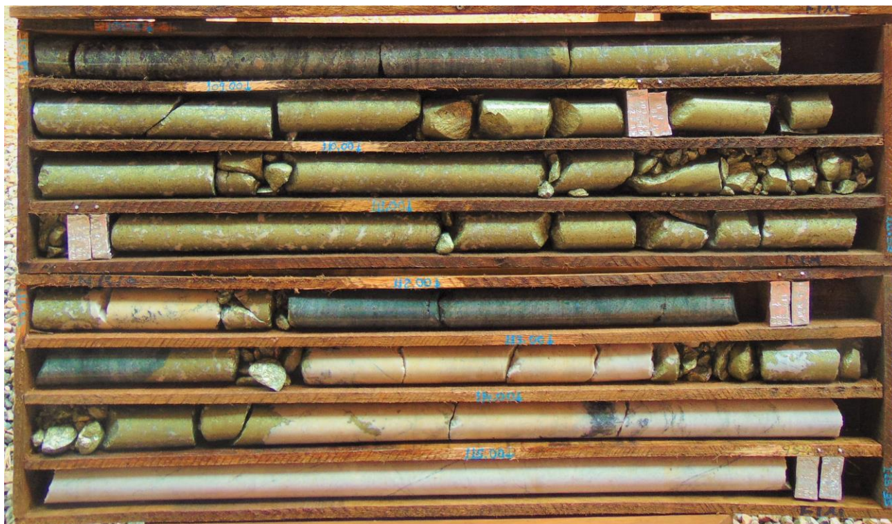
Figure 3: Core photo from drillhole ACLD-19-008, displaying the main copper sulphide mineralisation and alteration intersected in recent drilling
