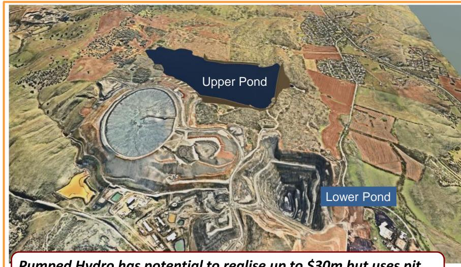
Pumped Hydro has potential to realise up to \$30m but uses pit as lower pond which limits underground mine life below pit
