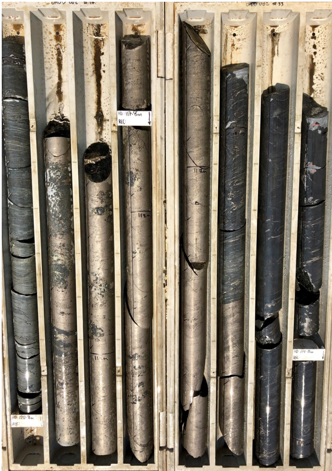
Figure 7: Massive sulphides in the Lower Zone of CHDD002 with 116.4m-120m grading 1.0% Cu, 4.9 g/t Ag
