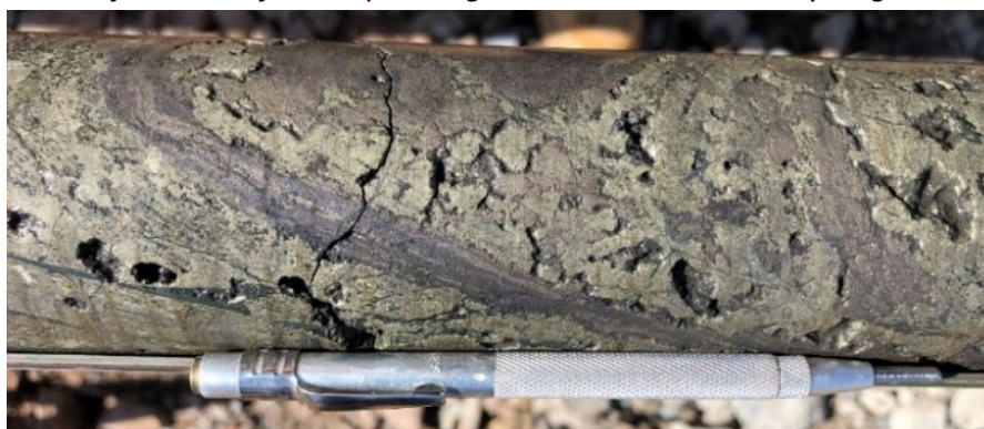
Figure 1: Massive sulphide from CHDD001 61.4m-61.9m grading 6.0% Zn, 0.7% Pb, 0.2% Cu, 14.1 g/t Ag.
