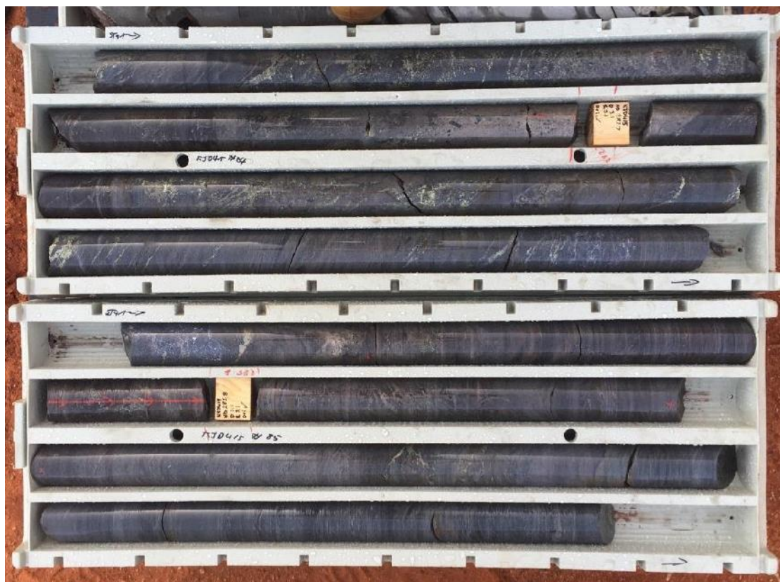
Figure 6 Photo of core from KJD415, showing mineralised interval from 274 to 281m
