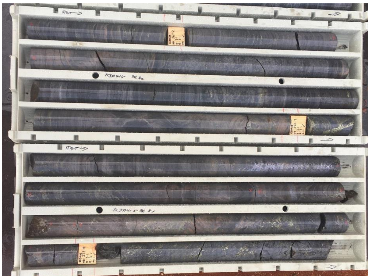
Figure 5 Photo of core from KJD415, showing mineralised interval from 266.7 to 274m
