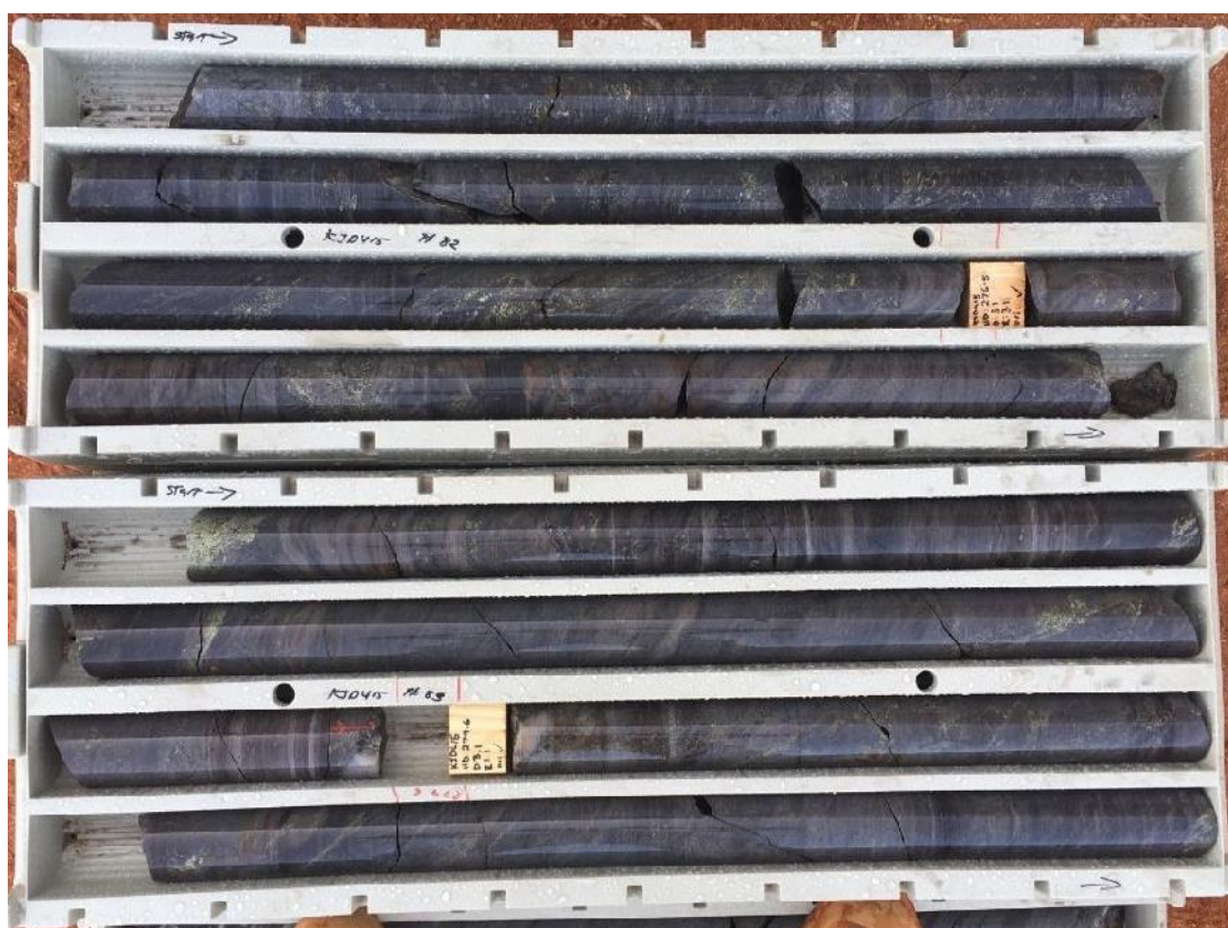
Figure 7 Photo of core from KJD415, showing mineralised interval from 281 to 287m
