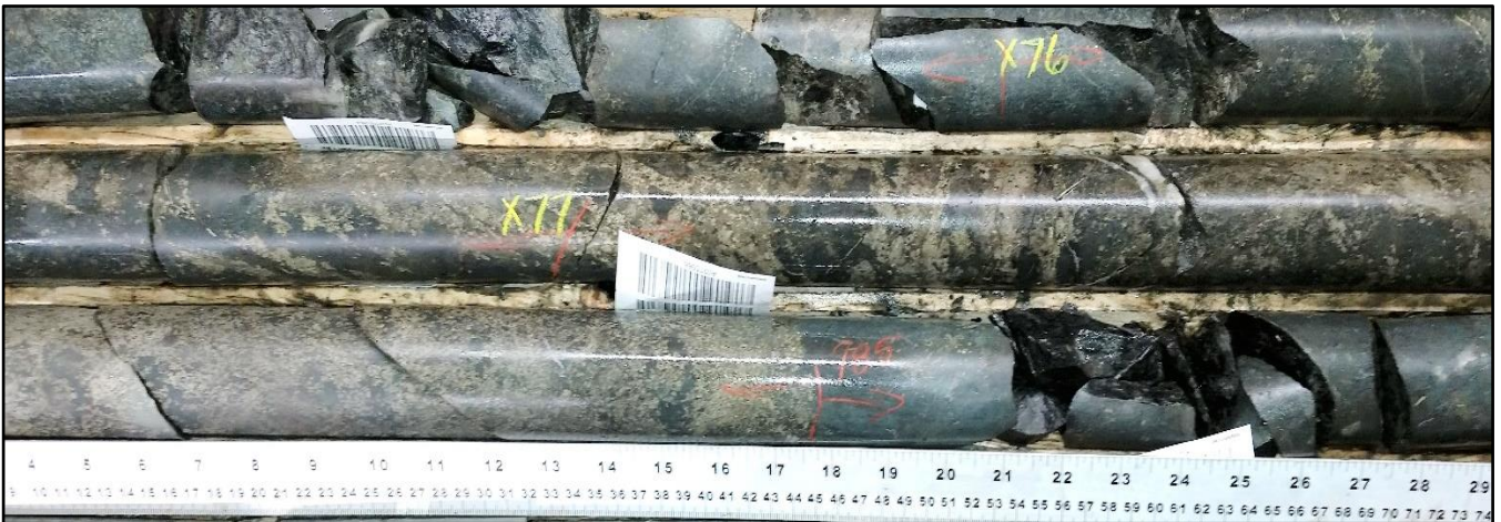
Figure 8: ZA-19-06 - footwall gabbro with semi-massive and net-textured pyrrhotite + pyrite at 76 to 78.5m downhole Assayed 2.5m at 1.3% Ni, 1.9% Cu, 1.0g/t PGE and 7g/t Ag.
