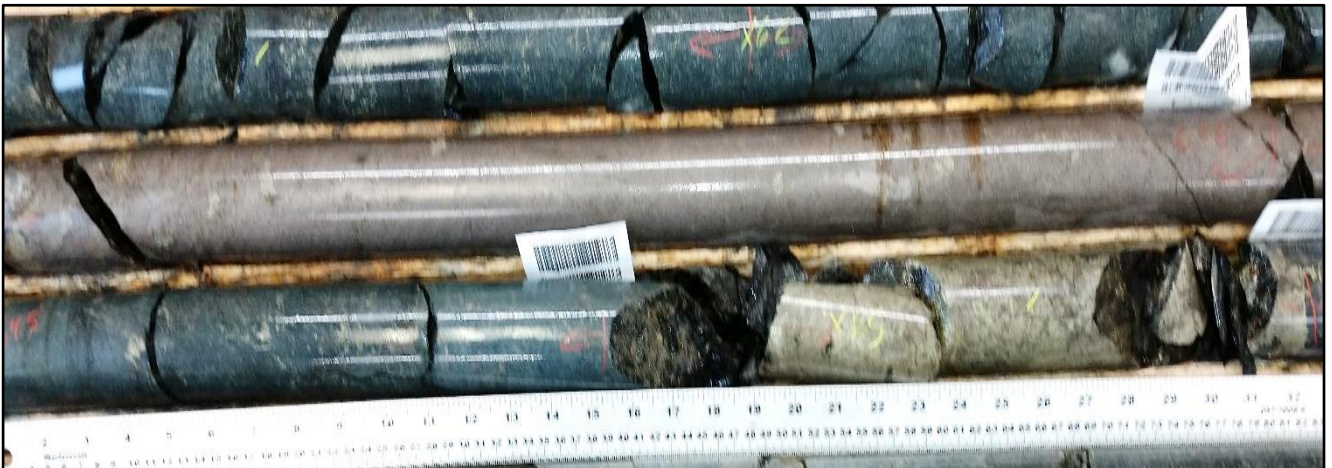
Figure 9: ZA-19-08 massive pyrrhotite with 5-10% pyrite at 63 to 64.5m downhole assayed 1.5m at 1.3% Ni, 0.9% Cu, 1.9g/t PGE and 2g/t Ag.
