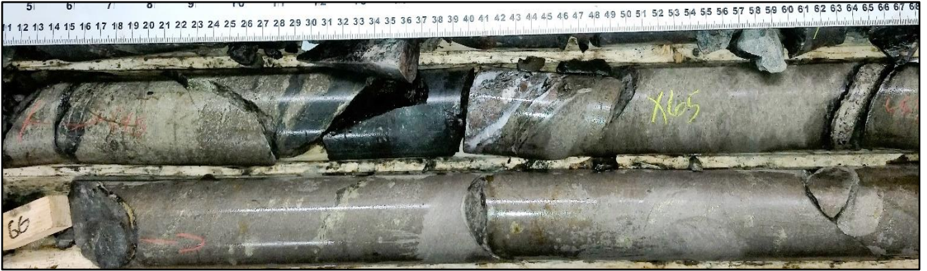
Figure 7: ZA-19-06 - massive sulphide comprising 95% pyrrhotite and 5% chalcopyrite at 65.2 -67.0m downhole. Assayed 1.8m at 2.1% Ni, 2.7% Cu, 2.3g/t PGE and 7g/t Ag.
