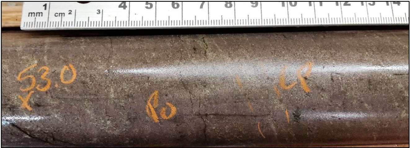
Figure 2: ZA-19-04 massive sulphide comprising pyrrhotite with bands of wispy chalcopyrite. Interval 53 to 54m assayed 1.0m at 2.64% Ni, 2.0% Cu and 2.8g/t PGE
