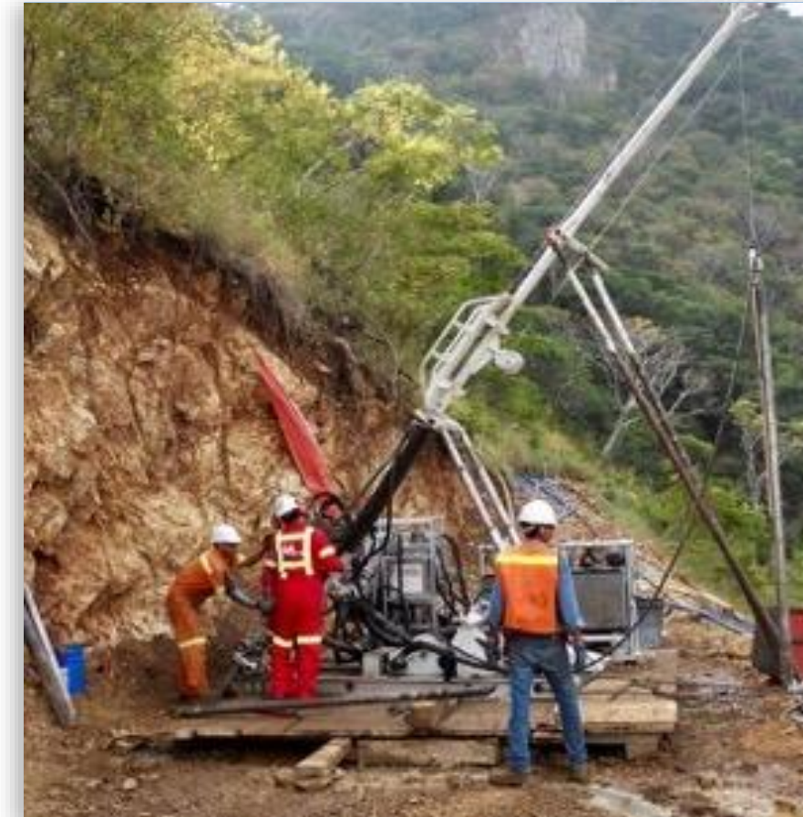
Type of diamond core drill rig to be used at Copalquin.
