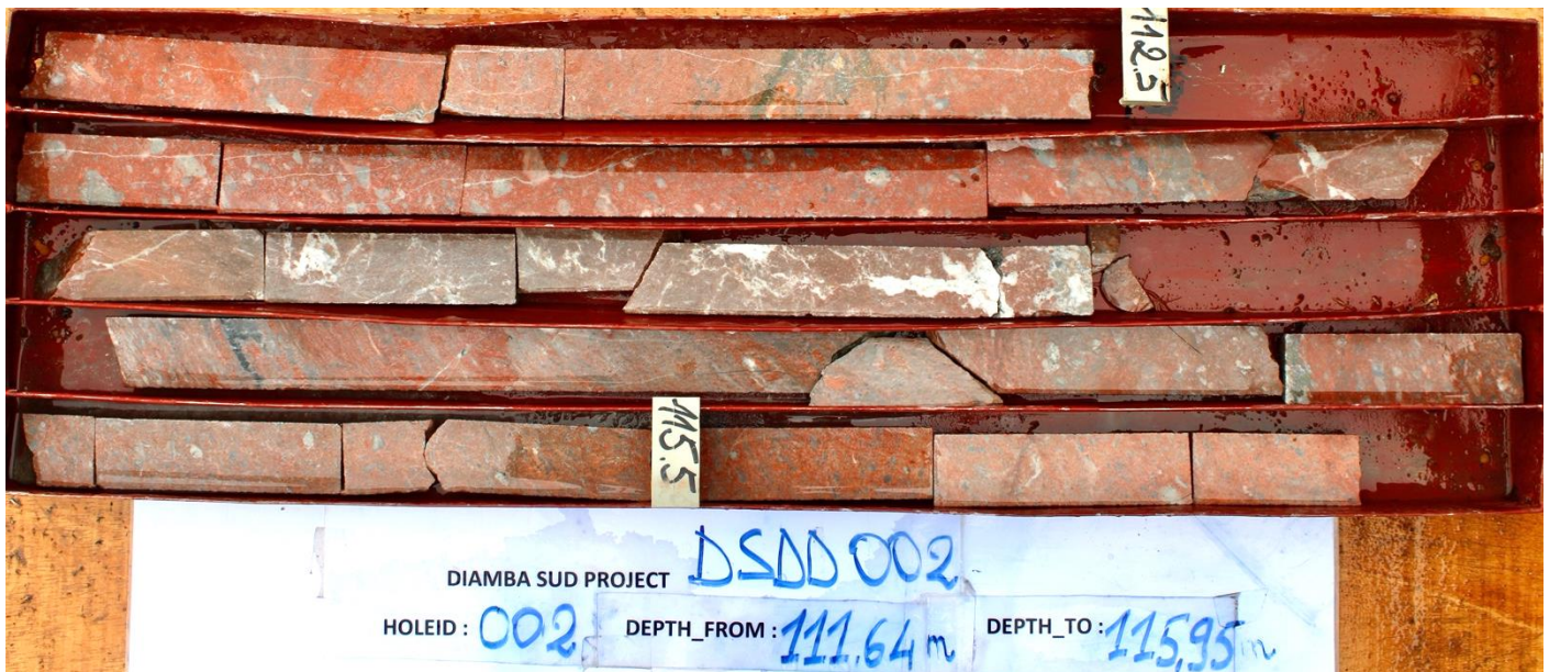
Figure 4: DSDD002,111.64-115.95m showing strongly altered felsic intrusive, with hydrothermal brecciation Pyrite mineralisation and quartz carbonate veining.
