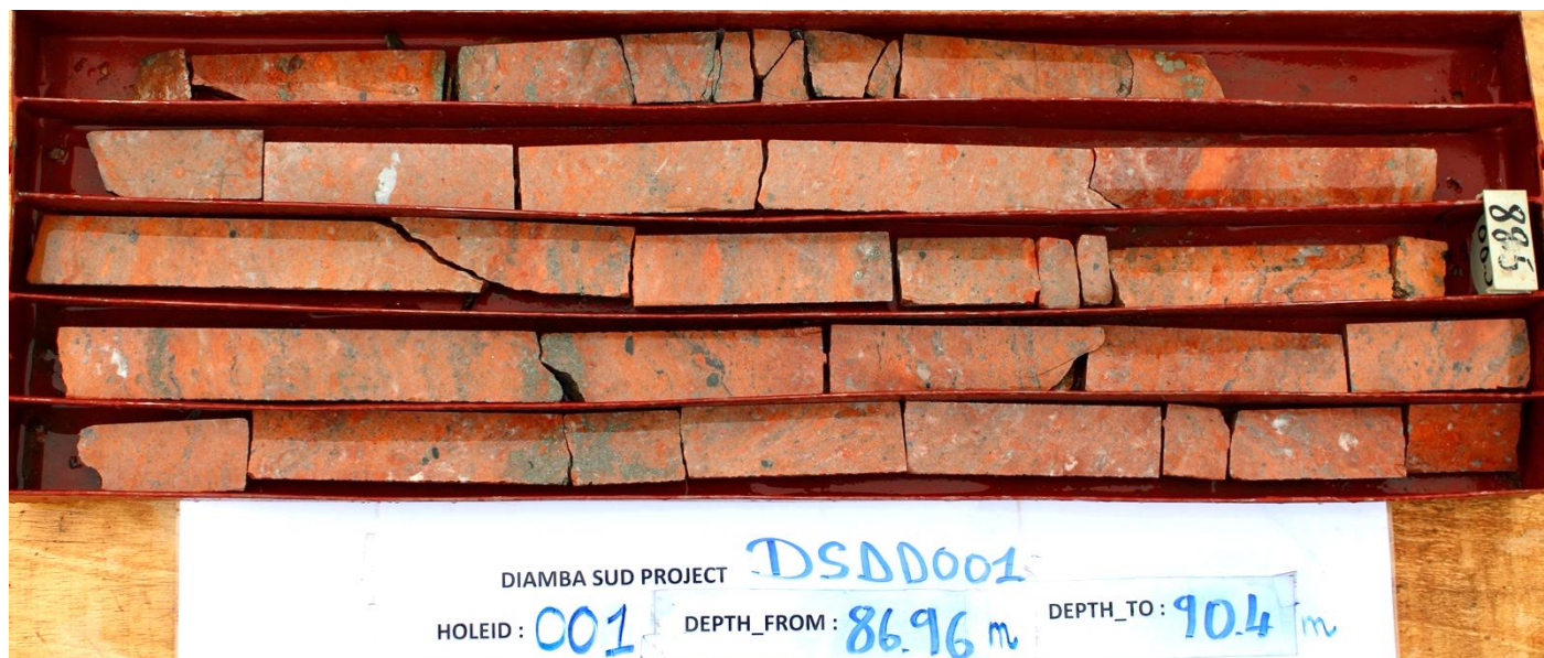
Figure 2: DDH001-86.96 to 90.4m, showing hydrothermal brecciation, strong alteration with foliation parallel/veinlets of coarse pyrite/qtz/carbonate infill and coarse disseminated pyrite.
