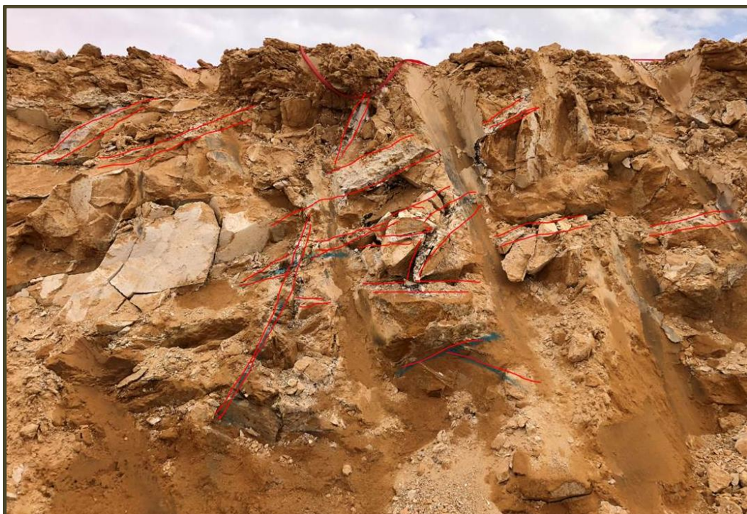
Figure 2: Quartz vein stockwork exposed in pit bench within supergene ore domain (approx. 4m wide area)
