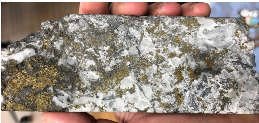
Figure 1: Highly mineralised section of drillcore from GRDD001 ~40.5m down hole depth which was part of the 40.3m-40.7m interval which graded 9.1% Cu, 0.9 g/t Au, 1.6 g/t Ag and 0.1% Co.
