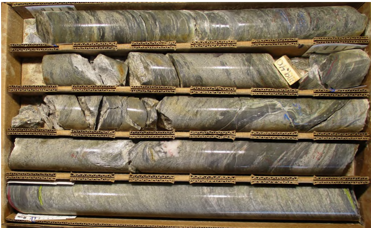
Figure 6: Massive sulphide mineralised interception at hole BMZ79 from 417.3 metres to 420.28 metres downhole depth. Sulphide mineralisation both follows cross-cut primary foliation in the hosting rhyolite rock. Sphalerite is pale brown; chalcopyrite bright yellow. Pyrite completes the visible sulphide assemblage
