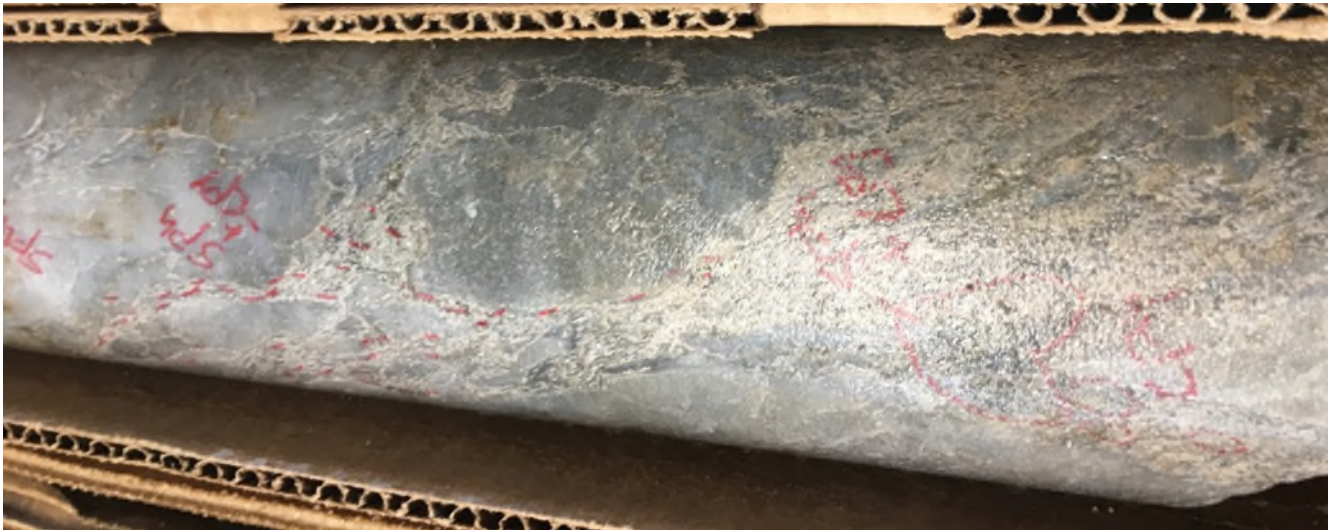
Figure 4: Closer view of Massive sulphide mineralised interception at hole BMZ80 at 408 metres downhole depth. Sulphide mineralisation both follows cross-cut primary foliation in the hosting rhyolite rock. Sphalerite is pale brown; chalcopyrite bright yellow. Pyrite completes the visible sulphide assemblage
