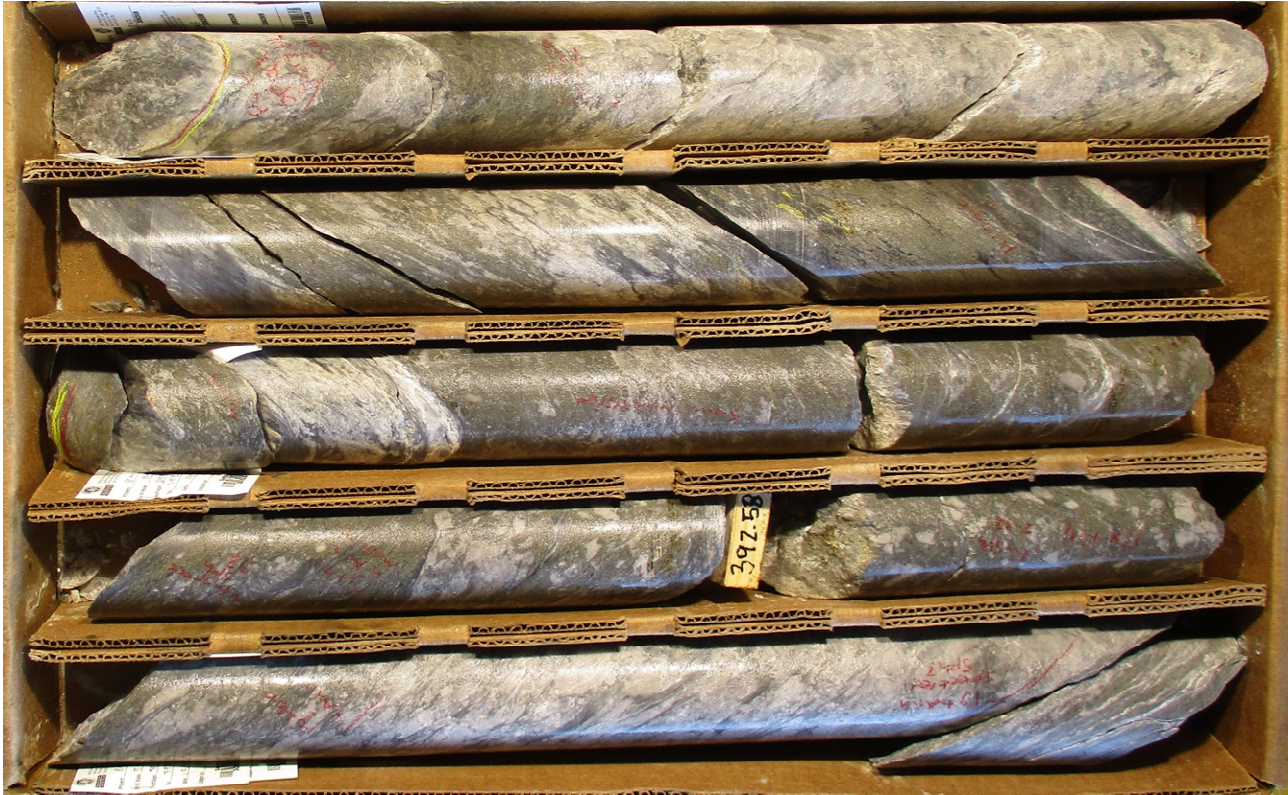
Figure 3: Massive sulphide mineralised interception at hole BMZ80 from 391.88 metres to 394.37 metres downhole depth. Sulphide mineralisation both follows cross-cut primary foliation in the hosting rhyolite rock. Sphalerite is pale brown; chalcopyrite bright yellow. Pyrite completes the visible sulphide assemblage
