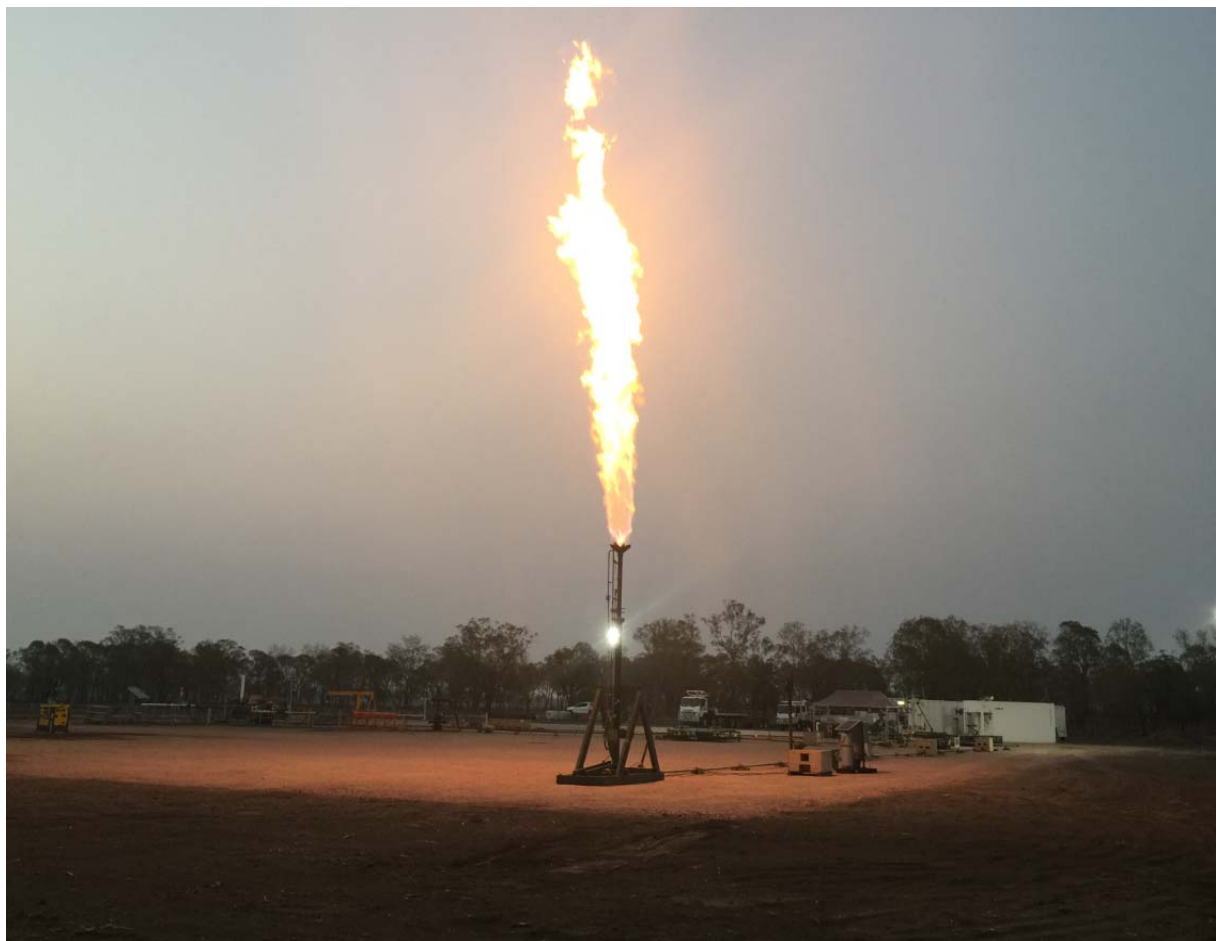
Myall Creek #5A– flaring initial gas of up to 4.4 MMCFD during flow back operations (photo taken at approximately 6pm 5 January 2020)
